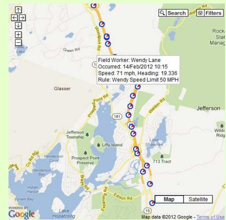
**Speed Trigger –** is a notification sent to administrator and/or employee if a rule is broken. Example is if management does not want company vehicles traveling over 70 mph an email and/or text message could be sent to driver to slow down and management that a speed rule was broken by that individual.
